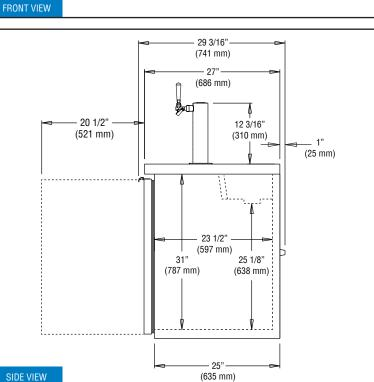
**IMPORTANT NOTE:** Models are completely front breathing and take in and exhaust air through the front grill. For proper operation, the area in front of the cabinet **must** not be obstructed in any way. A clearance of 1" on the back and 3" on the sides is recommended.
