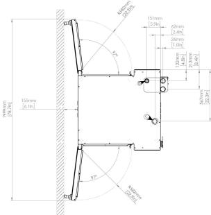
Notes to drawings: 400 mm / 15.75 inches spacing on right side of oven recommended for service access. Foot shown in standard and extended lengths.
