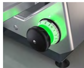
Gauge plate closed, safe for cleaning - green.
