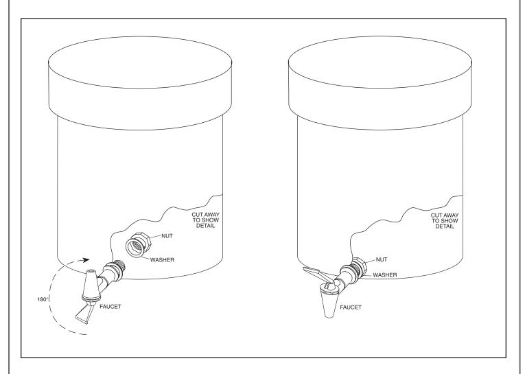
Make sure the spigot with washer is flush with the unit. Position the spigot upside down. Take nut with washer and screw on the end of the shank until hand tight. Continue to hold nut and turn spigot to the right until it is in its normal vertical position (180°).
