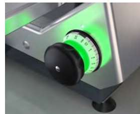
Gauge plate closed, safe for cleaning - green.
