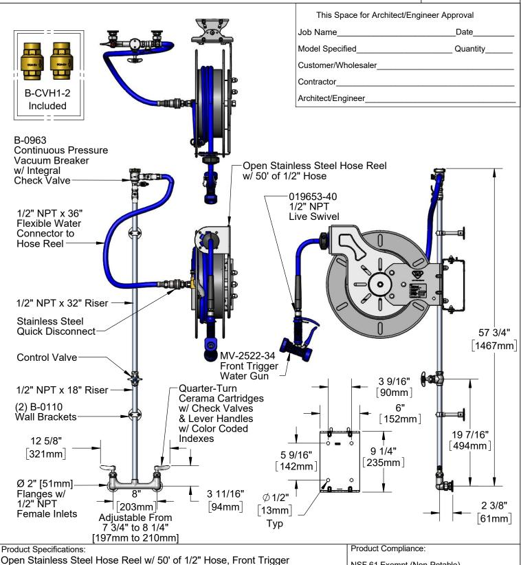
Water Gun w/ Swivel, 1/2" NPT Vacuum Breaker, 1/2" NPT Flexible Water Connector, 8" Wall Mount Mixing Faucet, Control Valve,
