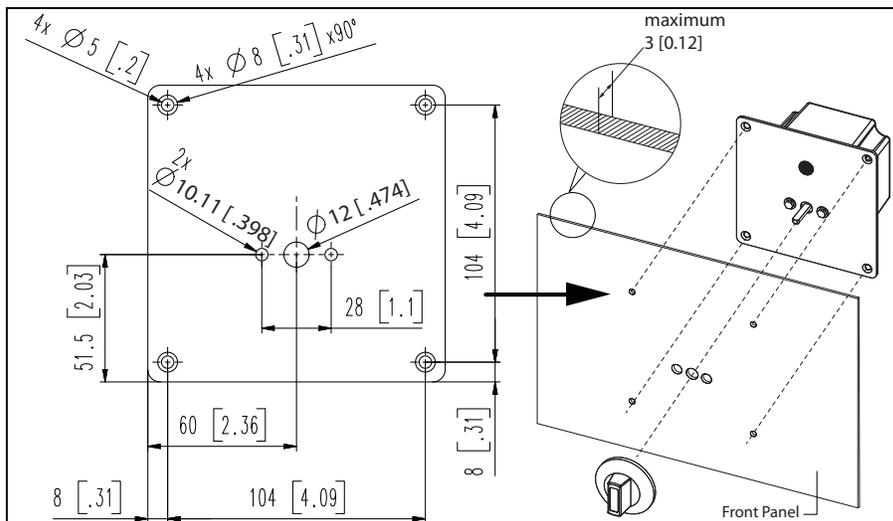
**To mount the control unit from the back of the panel:**
