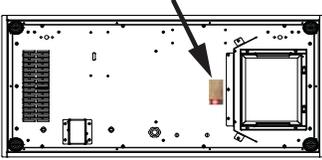
The rating plate specifies important information such as model number, serial number, and electrical specifications. The rating plate is affixed to the bottom of the unit, next to the air intake and air deflector.
