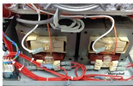
2000W e2s variant: two high voltage transformers side by side. Note: the left hand transformer supplies the right hand microwave circuit
