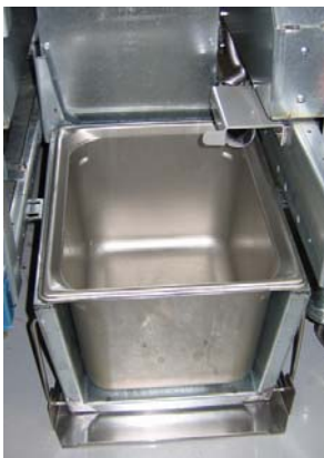
Figure 3: Insert the inner oil reservoir pan into the melting unit.
