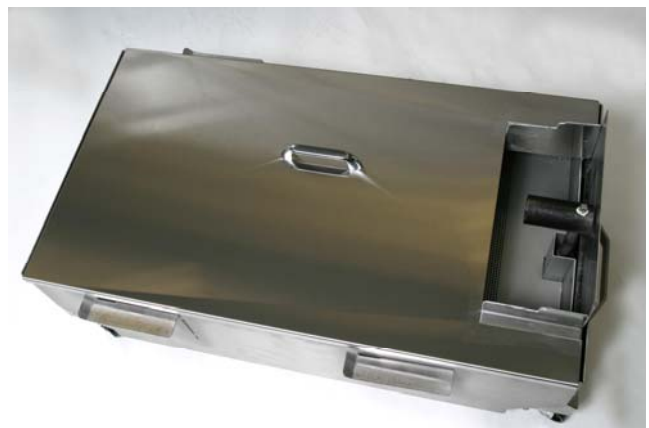
Fully assembled pan with pickup tube properly positioned in pan lid access hole. Position may vary between models.
