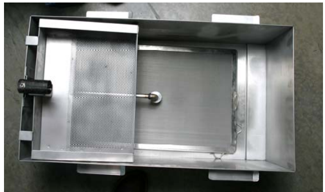
Crumb screen properly placed in filter pan.
