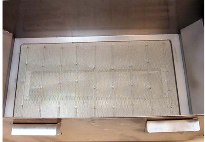
Support grid properly placed in filter pan.
