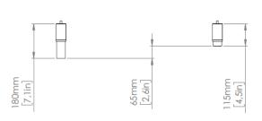
Notes to drawings:  $400~\mathrm{mm} \, / \, 15.75$  inches spacing on right side of oven recommended for service access.
