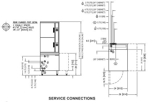
(7) – ELECTRICAL CONNECTION: 1/2" (13 mm) conduit connection to controls.
