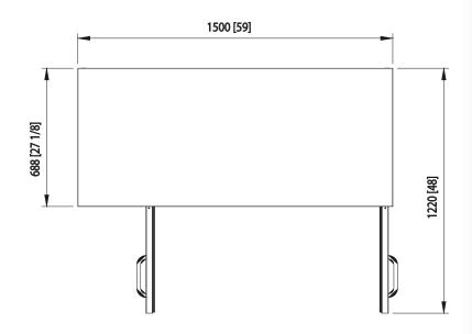
2 Door Capacity 19 Cu.Ft. Shelves Refrigerant R-290 Temperature 33°F ~ 39°F Range Easy Sliding Maintenance Condensing Unit 9.8 ft long (3m) flexible three Connection wire cord with modeled plug HP 3/8 Voltage 115V/60Hz **Amps** 3.8 NEMA Config. NEMA 5-15 Lighting Interior LED lighting
