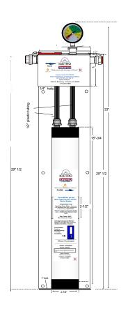
All IcePro cartridges should be changed out every six months or when there is a reduction in water pressure. Filter life depends greatly upon the quality of water. This product is for commercial use only and must be installed and maintained according to manufacturers guidelines www.icetroamerica.com or the warranty can be voided.
