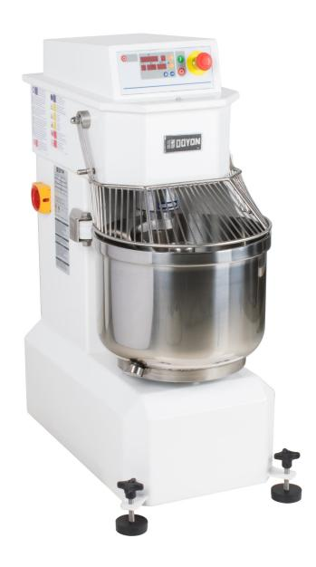
Spiral Mixer, 88 Lb. Dough Capacity, 2 Speeds, Programmable Digital Control, Stationary Stainless Steel Bowl, Safety Guard & Dough Hook, Cast Iron Frame with Enamel Coated Steel Finish, 4 HP, 208-240/60/1P/10A, NEMA 6-20P
