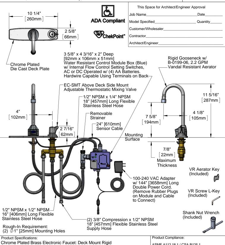
Chrome Plated Brass Electronic Faucet: Deck Mount Rigid Gooseneck w/ 8" Centers Deck Plate, Above Deck Side Mount Adjustable Thermostatic Mixing Valve w/ Integral Check Valves, AC/DC Control Module with Internal Flow Control Setting Switches, 18" Long Hot & Cold Supply Stop Flexible Connector Hoses
