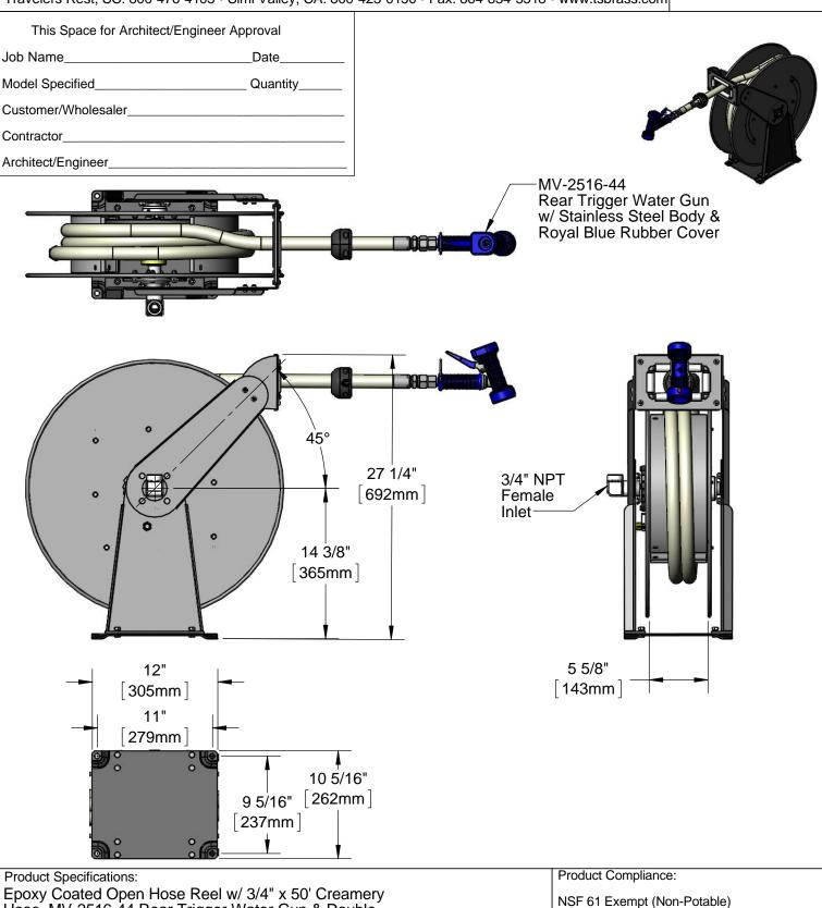
Hose, MV-2516-44 Rear Trigger Water Gun & Double Arm Support
