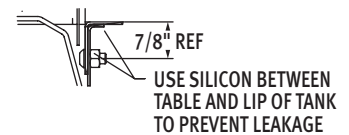
Sectional View Showing Table Connections
