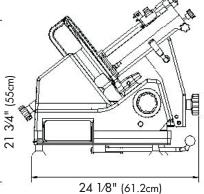
Controls: Manual slice thickness knob, digital membrane control for speed, stroke, and counter, removable blade sharpener
