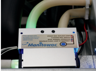
Manitowoc and Koolaire Luminice kits are not interchangeable. Luminice II will work with all "KT" models made after July 2017.
