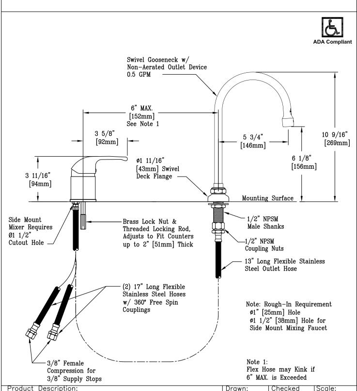
Side Mount Faucet: Remote Control Base w/ Flexible Stainless Steel Water Connectors, Cerama Cartridge, Swivel Gooseneck &
