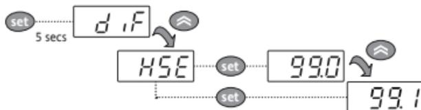
Select the desired parameter using the **▲** and **▼** keys. Press **set** to see the current value of the selected parameter. Press **▲** and **▼** to change the value and then press **set** to save it.
