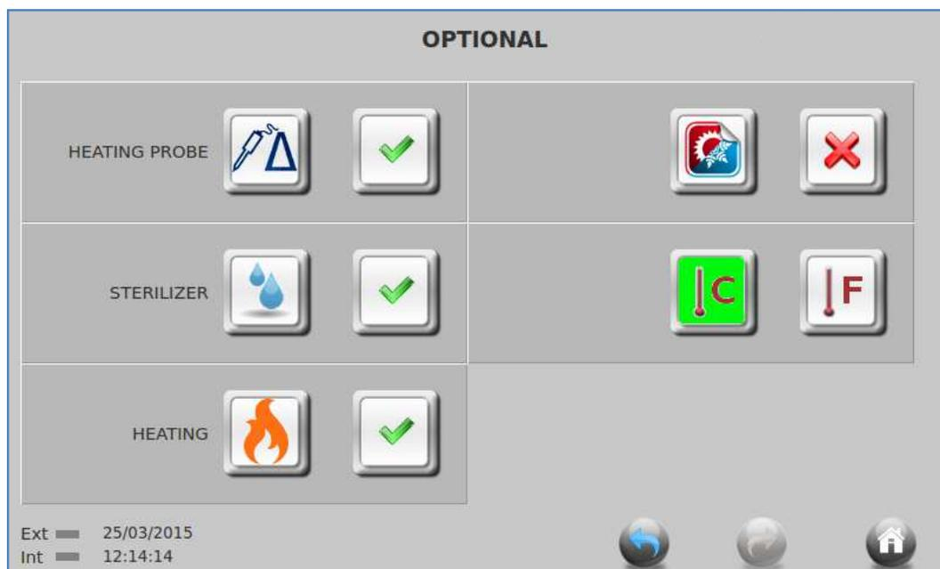
This menu will allow to enable or disable some advanced function such as: Core probe heating function, Sterilizer, Heating functions (left side) or Blast freezing cycle, temperature display mode, Celsius [°C] or Fahrenheit [°F].
