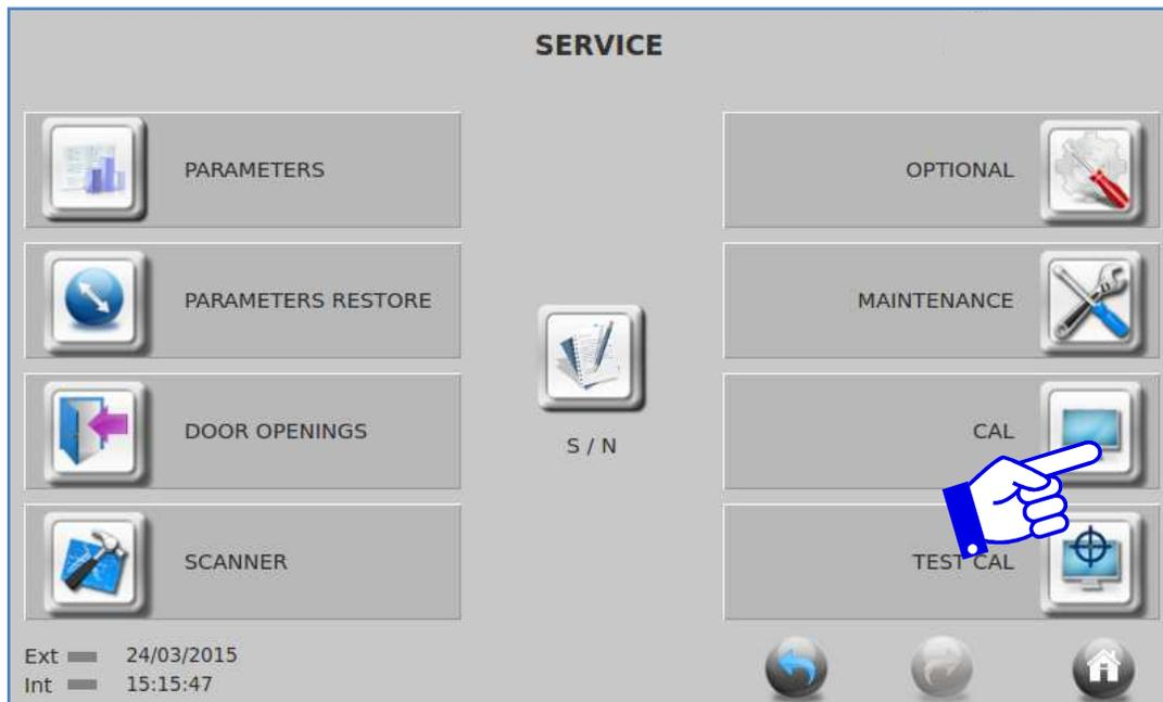
Press on the CAL tab, locate the red cross in the upper left hand corner and push on it, the cross will move to the upper right hand corner, push there and then to the lower left hand corner, push there and finally to the lower right hand corner, push there. Push then on the green checkmark to, the calibration is completed.
