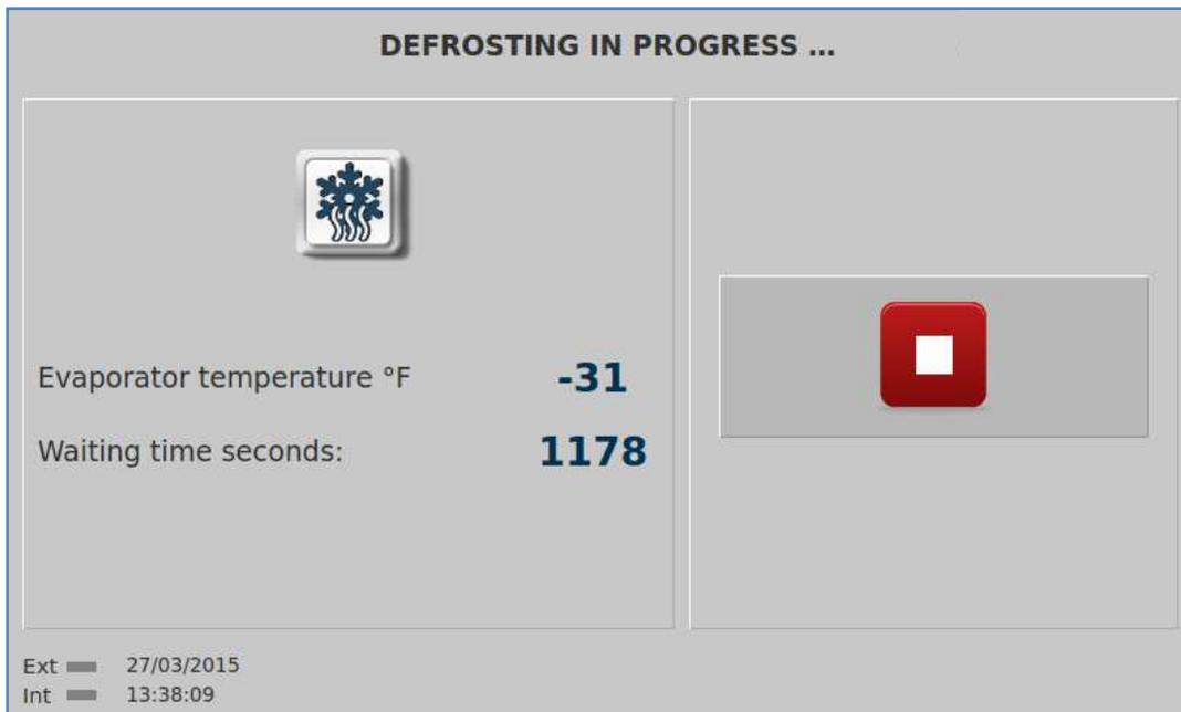
This is an air defrost cycle, so the fans will run at high speed. Once the Manual Defrost is complete by either time or temperature, the screen will return automatically to the Home screen or it can be terminated at any time by pressing the red stop button.
