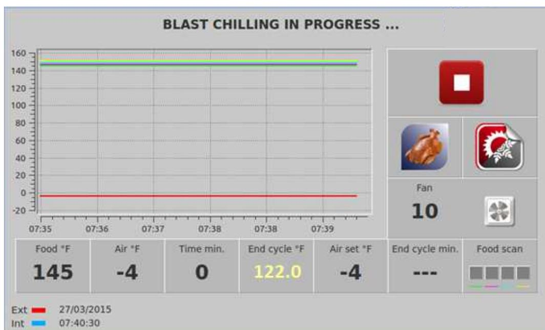
A graph will show in real time the food core temperatures read by the food probe and the air temperature. On the right side it will show the food under process, the type of cycle (chilling or freezing icon), the fan speed. On the bottom the screen will also show real time values as well as cycle setpoint values. From left to right:
