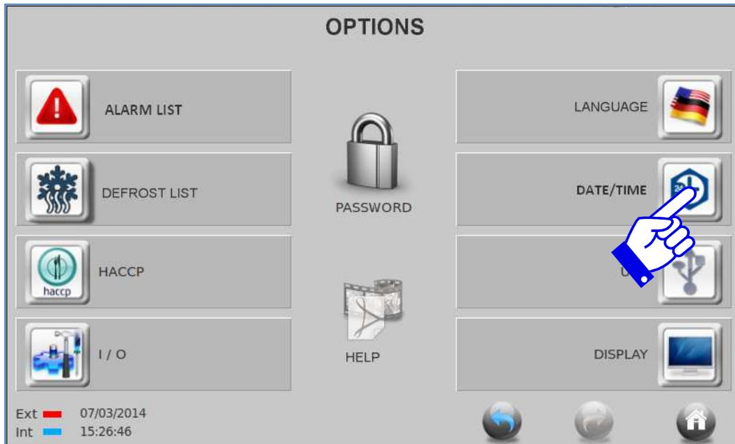
To set the proper date, firstly set the day, then the month and finally the year. Use the up and down arrows to reach the proper date and time.
