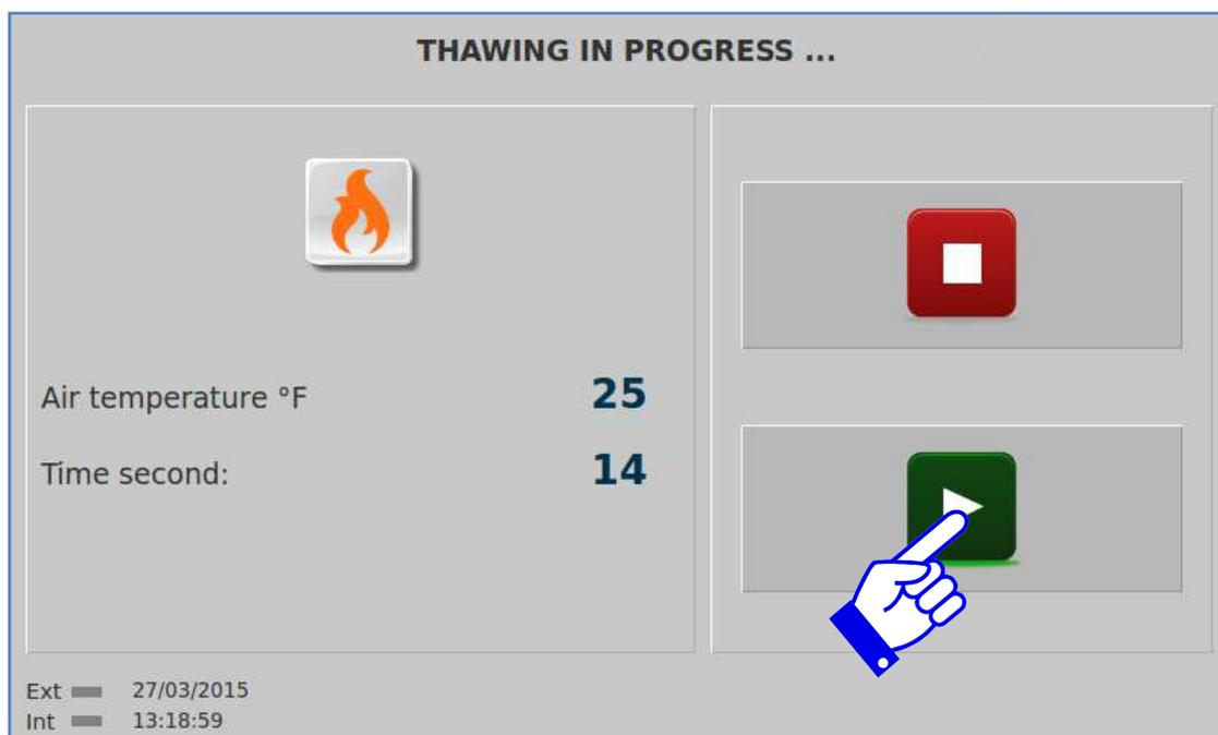
The air temperature can be set within 0°C(32°F) and 9°C(48°F). The insert probe can be also used to run a product temperature based cycle, hence obtaining a notification from the display when the product is ready to re-thermalize (i.e. 3°C-37°F). Or otherwise set a time based cycle to run the thawing process for a predetermined time.
