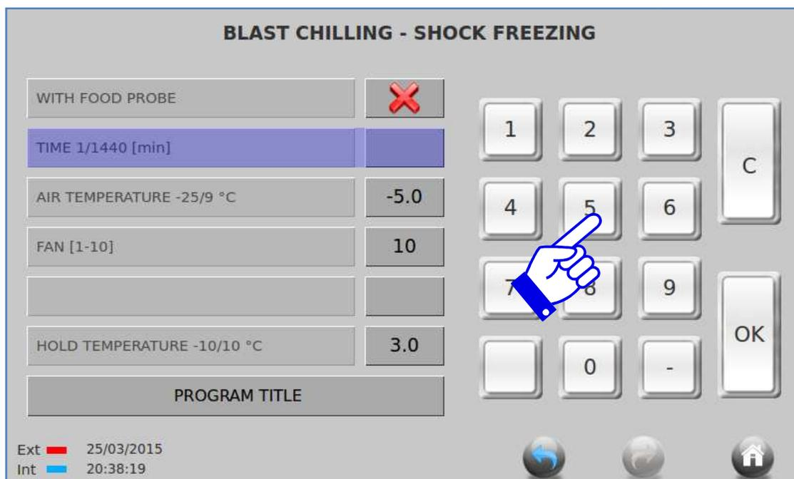
Using the key pad, select the correct number corresponding to the range indicated by each mode.
