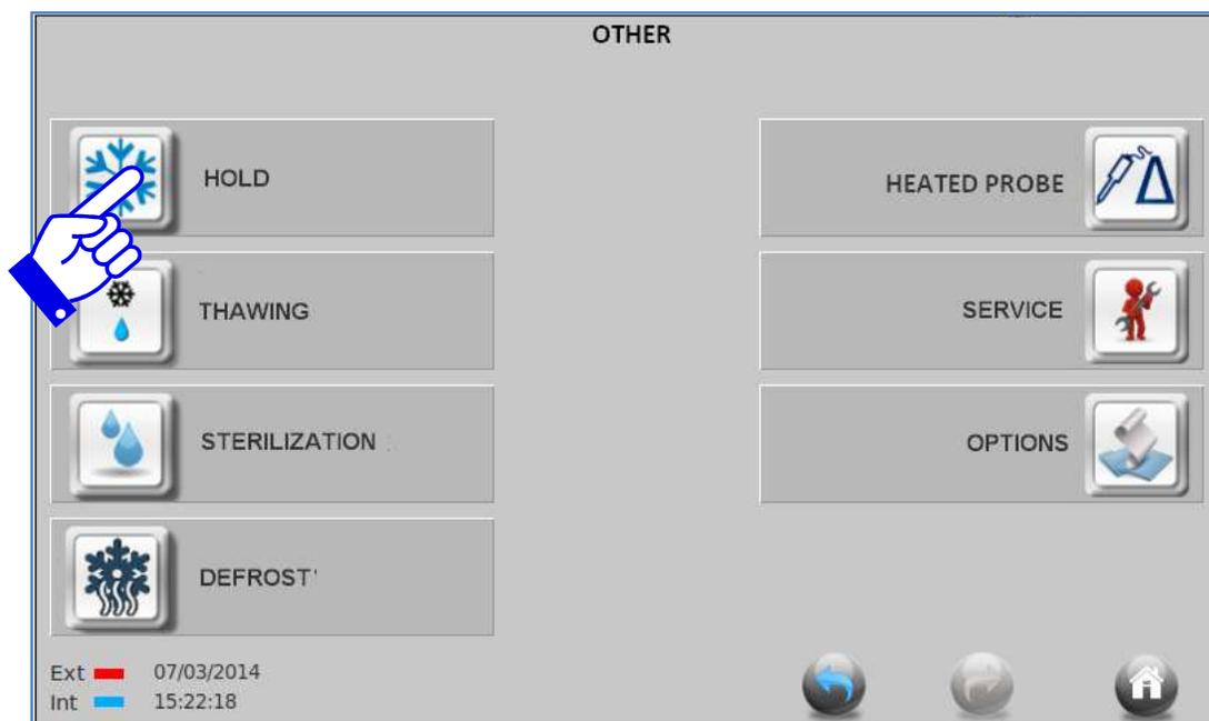
To change the hold temperature, press the Air temperature tab, the tab will turn blue and you can select a temperature from  $-40^{\circ}\text{C}$  ( $-40^{\circ}\text{F}$ ) to  $8^{\circ}\text{C}$  ( $46^{\circ}\text{F}$ ). If no temperature is selected or a temperature is selected outside of the range and start is pushed, the tab will turn red and not allow you to continue until a correct temperature is selected.
