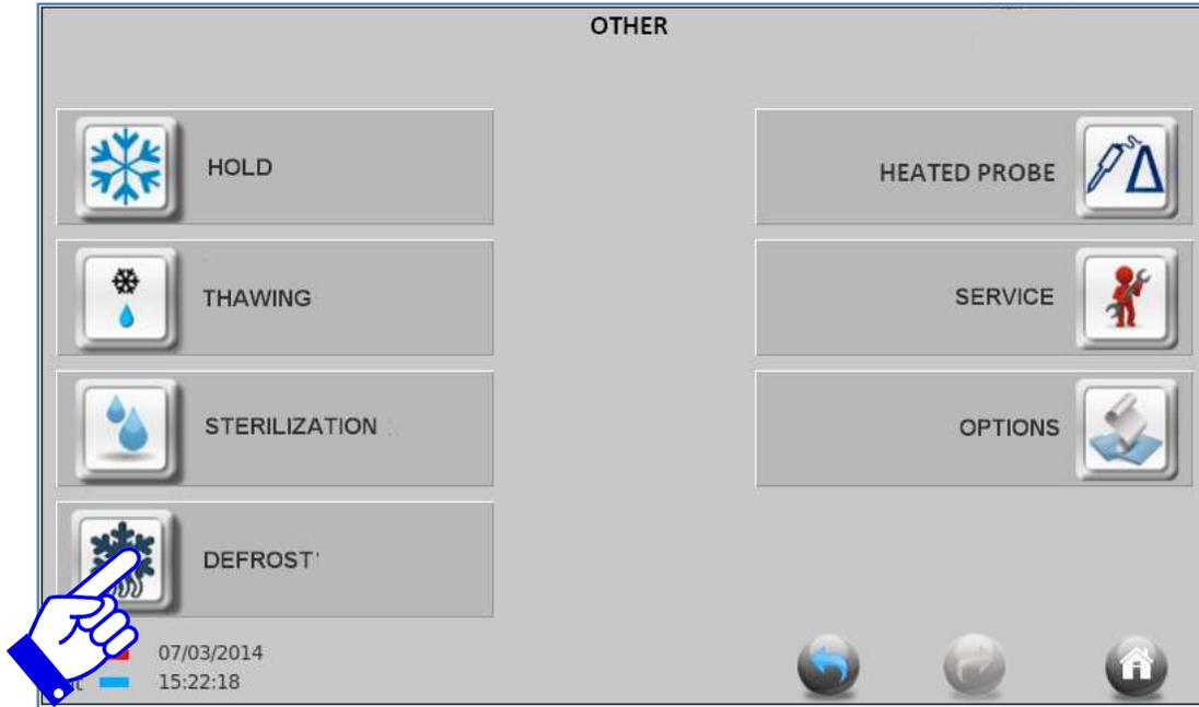
The Manual Defrost cycle is programmed to run for 10 minutes or until the evaporator temperature reaches 8°C(46°F).
