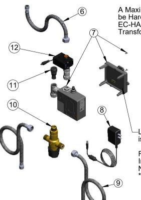
A Maximum of (8) ChekPoint Faucets can be Hardwire Connected and Powered by EC-HARDWIRE ChekPoint Hardwire AČ Transformer. (Sold Separately)
