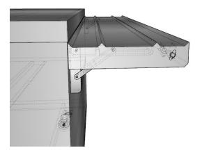
\*All serving counters will include connection latches at front and back for joining counters together. Along with the other offerings in the SPARTAN serving lineup, this allows for the creation of complete serving lines with interlocking counters in whatever configuration is required for the application.
