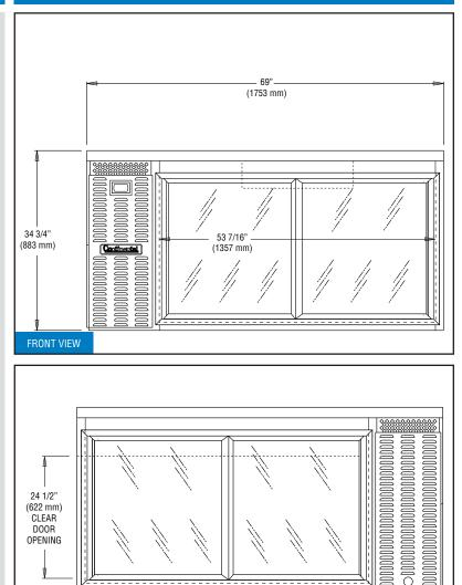
**IMPORTANT NOTE:** Models are completely front breathing and take in and exhaust air through the front grill. For proper operation, the area in front and back of the cabinet must not be obstructed in any way. A clearance of 3" on the sides is recommended.
