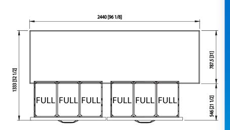
**Drawers** Capacity 21.4 Cu.Ft. Refrigerant R-290 Temperature 33°F ~ 39°F Range Easy Sliding Condensing Unit Maintenance 9.8 ft long (3m) flexible three Connection wire cord with modeled plug HP 3/8 Voltage 115V/60Hz **Amps** 3.5 **NEMA Config.** NEMA 5-15
