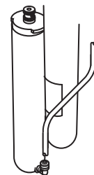
Remove the red SFC tubing from the fitting before completely removing the RO membrane cartridge
