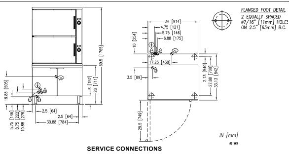
(1) - ELECTRICAL CONNECTION: Field wiring electrical connection to be as specified on data plate.
