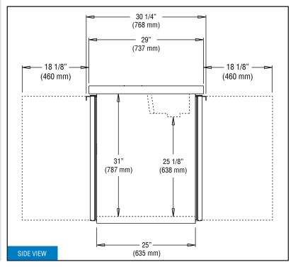
**IMPORTANT NOTE:** Models are completely front breathing and take in and exhaust air through the front grill. For proper operation, the area in front and back of the cabinet <u>must</u> not be obstructed in any way. A clearance of 3" on the sides is recommended.
