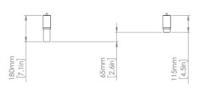
Notes to drawings: 400 mm / 15.75 inches spacing on right side of oven recommended for service access. Foot shown in standard and extended lengths.
