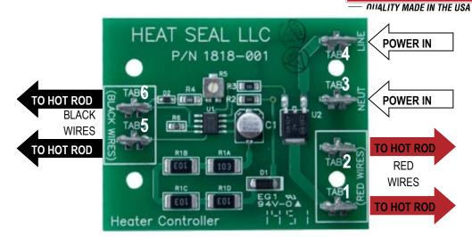
THIS UNIT SHOULD NOT BE OPERATED IF ROD TEMPERATURE EXCEEDS 300°F. IF SMOKE OR FUMES ARE DETECTED, DISCONTINUE USE
