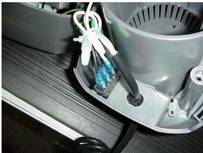
Figure 2. Cord and circuit breaker switch.
