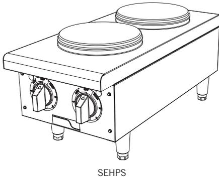
APW Wyatt electric hot plates will be constructed in the U.S.A. consisting of an aluminized steel with stainless top and front. Units are equipped with infinite controls, 2 indicator lights, and are available with incoloy sheath tubular elements or sealed ceramic elements. Hot plates have a junction box at the rear of the unit for electrical connection and operate on 208V or 240V. Units carry the approval of Underwriters' Laboratories, NSF listed and CSA approved.
