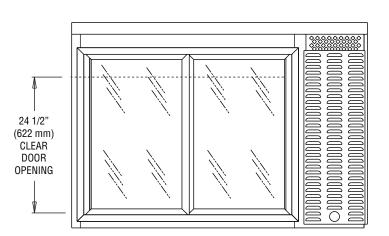
**IMPORTANT NOTE**: Models are completely front breathing and take in and exhaust air through the front grill. For proper operation, the area in front and back of the cabinet <u>must</u> not be obstructed in any way. A clearance of 3" on the sides is recommended.
