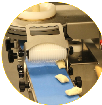
Optional guillotine cutting group, optional conveyor belt, and optional decorative rollers
