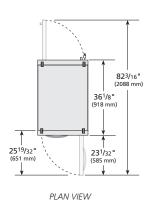
$Specifications \ subject \ to \ change \ without \ notice.$  Chart dimensions are rounded up to the nearest  $\frac{1}{6}$ " (millimeters rounded up to the next whole number).
