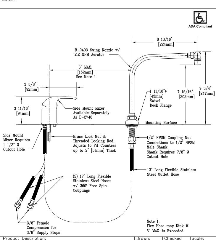
Side Mount Faucet: Single Lever Base Mixing Faucet w/ 3/8" Compression Female Flex Stainless Steel Supplies, Ceramic Cartridge & 9 3/4" High Swing Nozzle w/ 2.2 GPM Aerator
