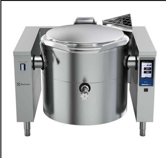
587041 (PBOT15GDWF) Touchline Tilting Kettle, gas, 40 gallon (150 Lt) capacity, stainless steel construction, full jacket, safety valve, safety thermostat, motor assisted tilt, 2" tangent draw-off valve, 88712 BTU
