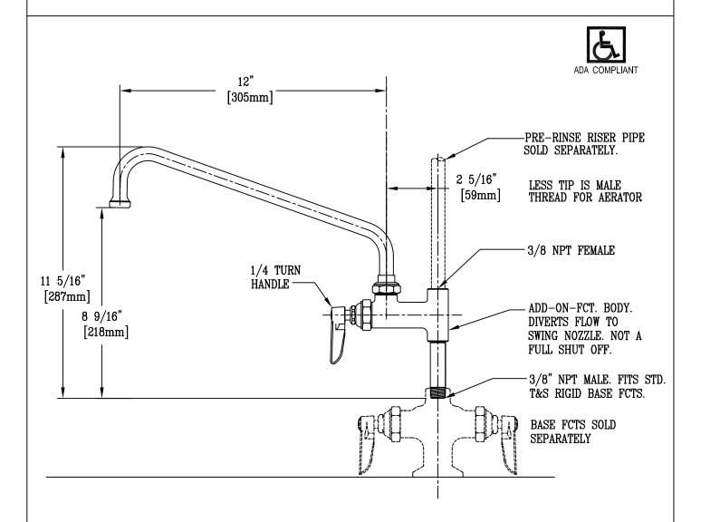
NOTES: 1. THE ADD-ON FAUCET IS AN ADDITION TO PRE-RINSE UNITS AND IS INSTALLED IN OUTLETS OF BASE MIXING FAUCETS OF UNITS BEFORE FITTING RISER PIPE, AS SHOWN.
