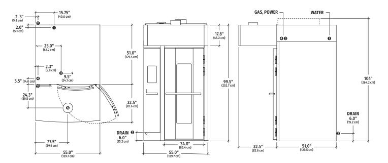
Highest Point on Oven: 104" (265cm) Rack Swing Diameter: 34.5" (87.6 cm) Shipping Weight: 3,443 lbs. (1562kg) (shipped whole)/3,218 lbs. (1460kg) (shipped split)
