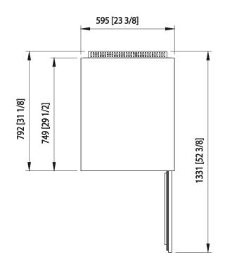
Door Capacity 7.9 Cu.Ft. Shelves Refrigerant R-290 Temperature 33°F ~ 39°F Range Sliding Easy Maintenance Condensing Unit 9.8 ft long (3m) flexible three Connection wire cord with modeled plug HP 1/4 Voltage 115V/60Hz 2.5 **Amps NEMA** Config. NEMA 5-15 Lighting Interior LED lighting
