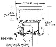
standard hose thread 3/4" GHT. Drain hose must be attached for unit to operate
