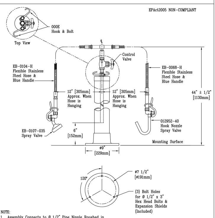
1. Assembly Connects to  $\emptyset$  1/2" Pipe Nipple Roughed in From Floor to a Height of 6"
