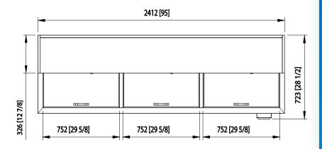
3 Doors Capacity 31.3 Cu.Ft. Dividers 5 Refrigerant R-290 Temperature 33°F ~ 39°F Range Sliding Easy Maintenance Condensing Unit 9.8 ft long (3m) flexible three Connection wire cord with modeled plug HP 3/8 Voltage 115V/60Hz **Amps** 3.5 NEMA Config. NEMA 5-15 Lighting Interior LED lighting
