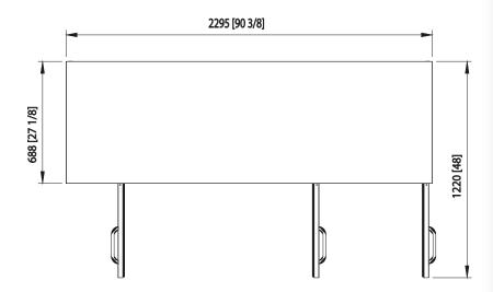
Door Capacity 31.5 Cu.Ft. Shelves 6 Refrigerant R-290 Temperature 33°F ~ 39°F Range Easy Sliding Maintenance Condensing Unit 9.8 ft long (3m) flexible three Connection wire cord with modeled plug 3/8 HP Voltage 115V/60Hz 3.8 **Amps** NEMA Config. NEMA 5-15 Lighting Interior LED lighting
