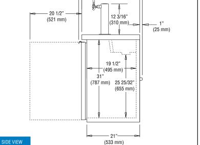
**IMPORTANT NOTE**: Models are completely front breathing and take in and exhaust air through the front grill. For proper operation, the area in front of the cabinet **must** not be obstructed in any way. A clearance of 1" on the back and 3" on the sides is recommended.
