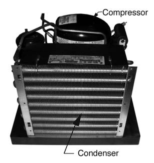
The condenser face can be cleaned with the use of a hose/brush attachment on a vacuum cleaner. Take care to avoid bending the condenser fins, It is of vital importance that the condenser gets the proper amount of air through the fins and around the tubes, therefore all dirt, lint, and dust needs to be removed.
