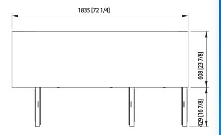
3 Doors Capacity 19.6 Cu.Ft. Shelves 6 Refrigerant R-290 Temperature 33°F ~ 39°F Range Easy Sliding Maintenance Condensing Unit 9.8 ft long (3m) flexible three Connection wire cord with modeled plug HP 3/8 Voltage 115V/60Hz **Amps** 3.5 NEMA Config. NEMA 5-15 Lighting Interior LED lighting
