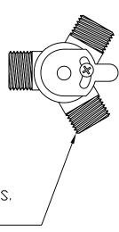
TEMPERATURE MIXING VALVE. ½" NPSM MALE (TYP 3 PL.) POLISH CHROME PLATED BRASS. INTEGRAL CHECK VALVES IN HOT AND COLD INLETS.
